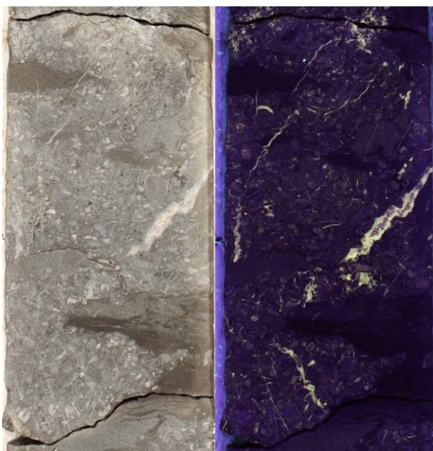
Figure 3. White light and UV photos of Wolfcamp A core from the Midland Basin. Preliminary results illustrate a complex history of diagenetic alteration and hydrocarbon migration.
