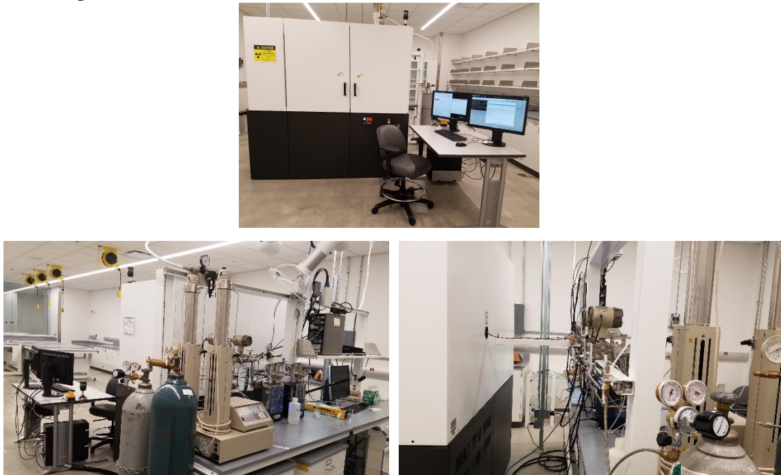
Figure 1. The University of Kansas's HeliScan micro-CT scanner and its integrated flow system
