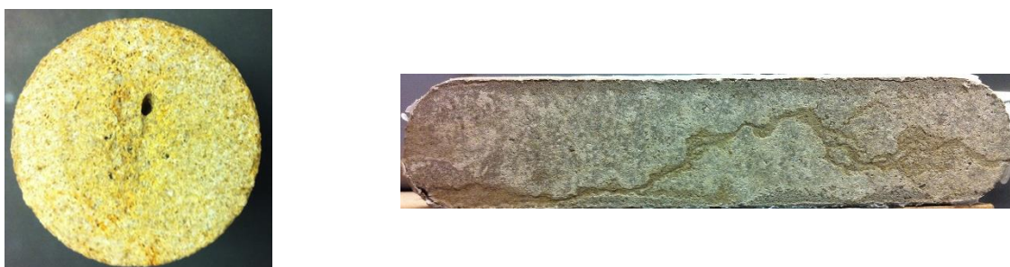
Figure 2. The LHS picture presents a core sample after a matrix acidizing experiment is performed. The RHS picture is a core sample after an acid fracturing experiment was performed.
